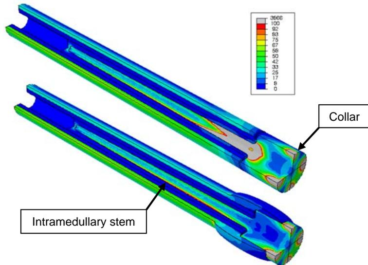
**Figure 1: (top) Von mises stresses with 0% osteointegration (bottom) Von mises stresses with 75% of the collar integrated**
