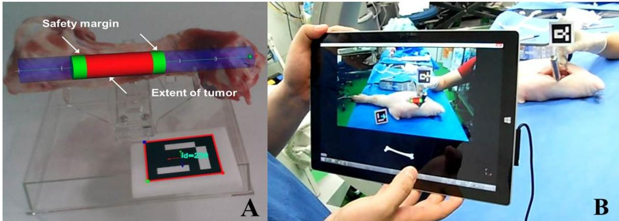
Fig. 1. (A) Cylinder-shaped virtual template. (B) AR-based navigation run on a tablet PC.
